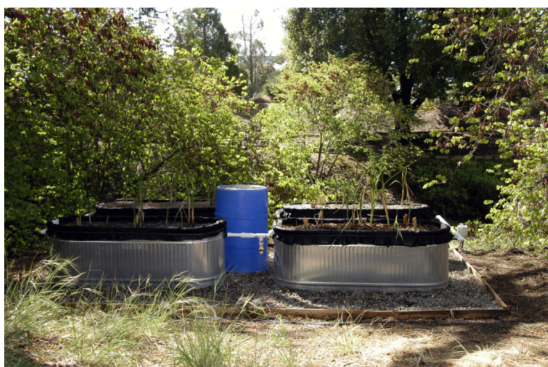
Water from the Arboretum waterway circulates through four basins in sequence in an experimental filtration system that mimics a natural wetland. The project is part of the graduate research of student Amelia Holmes, working with Professor of Civil and Environmental Engineering Jeannie Darby (see Constructed Wetland, opposite).
